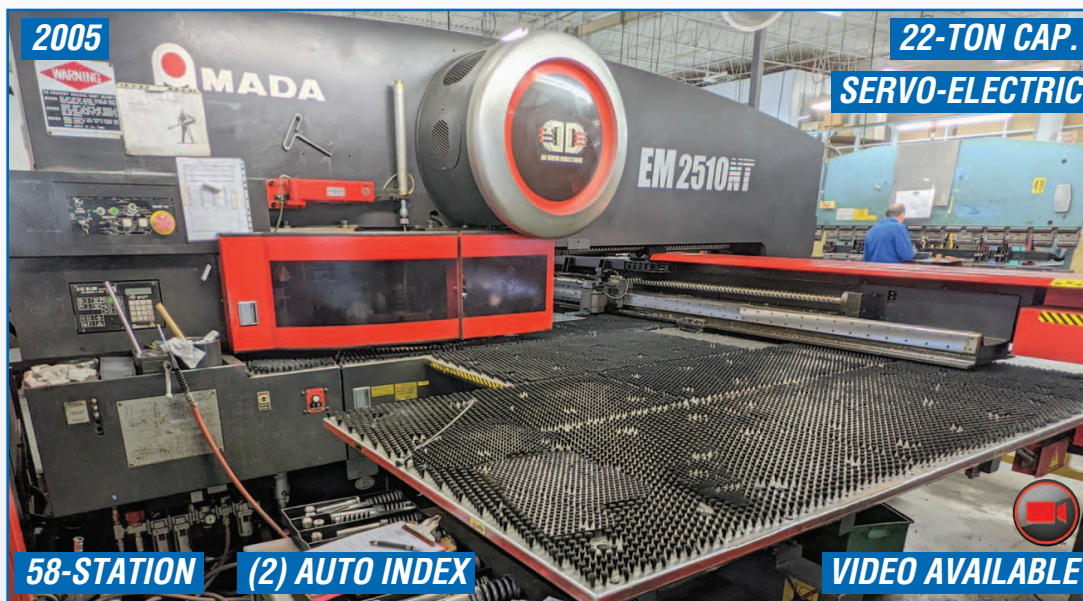
AMADA EM2510NT SERVO-ELECTRIC CNC TURRET PUNCH
